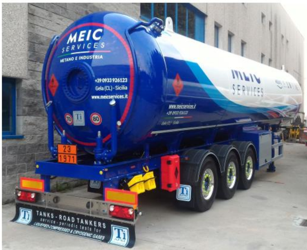
Figure 9: Self-carrying road tanker for CNG transportation
