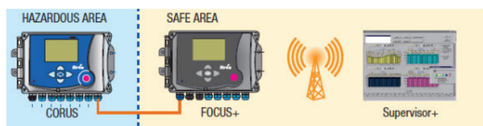
Figure 2. Data collection with VC modem
