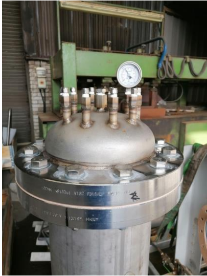
Fig. 2: Larger, 50-litre pressure vessel, designed for up to 45-50-bar operation, with fed-batch upgrade achieving up to 6 Nm 3 /hr at 0.11 kWhr/Nm 3 at circa 15-18 bar g.
