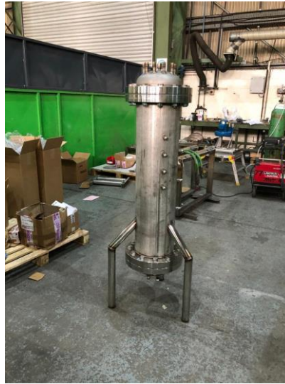
Fig. 2: Larger, 50-litre pressure vessel, designed for up to 45-50-bar operation, with fed-batch upgrade achieving up to 6 Nm 3 /hr at 0.11 kWhr/Nm 3 at circa 15-18 bar g.
