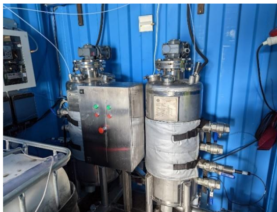
Image 2 Pilot-scale digesters –Test (treated with GasAbate) vs. Control (untreated)
