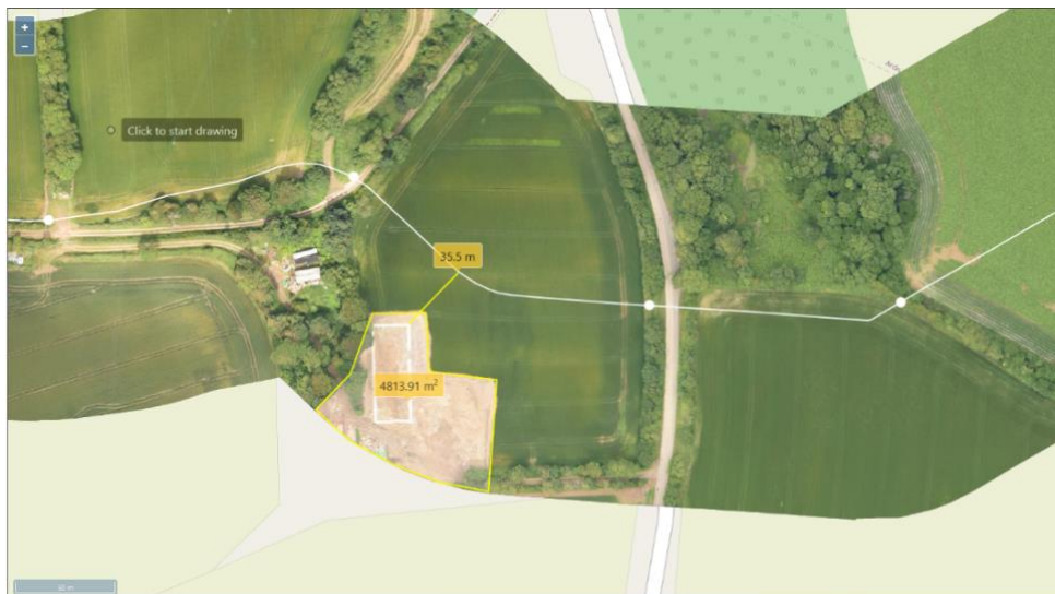
Figure 13: Aerial survey data (orthomosaics) enables precise measurements of objects captured in the imagery
