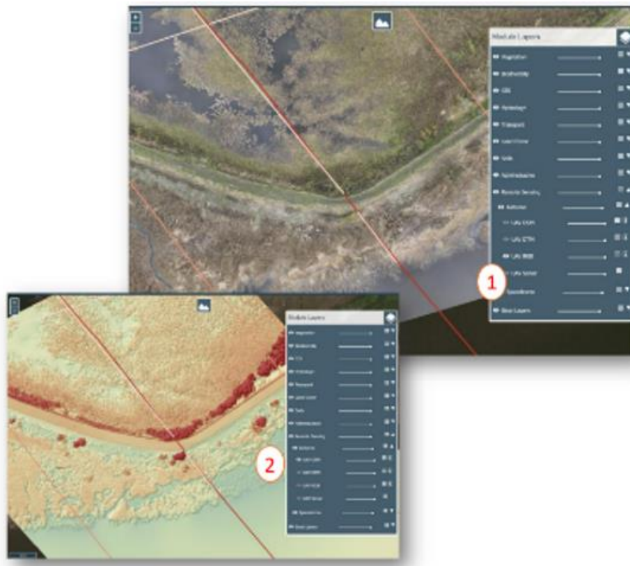
Figure 17: Topographic information of the River Shannon embankments; imagery (upper image) and DSM (lower image) accessible through the GNI prototype data platform
