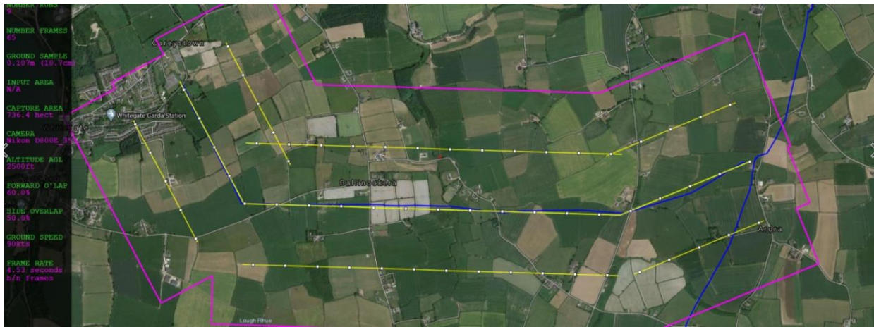
Figure 8: Aerial survey aircraft flight lines over a section of the pipeline in East cork – the aircraft follows a predetermined flight path to ensure that data is collected for the entire pipeline and surrounding environment
