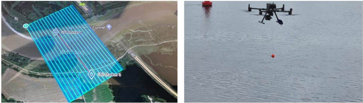
Figure 15: Flight profile over river crossing (left image) and sonar device ('orange' ball shaped object) deployed under drone (right image)
