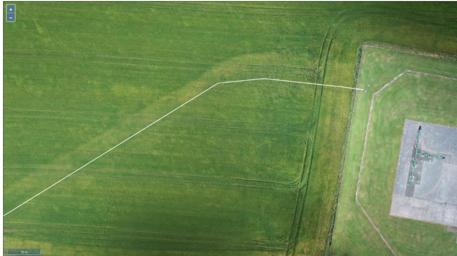
Figure 14: Aerial survey data (orthomosaics) enables reinstatement works to be clearly identified
