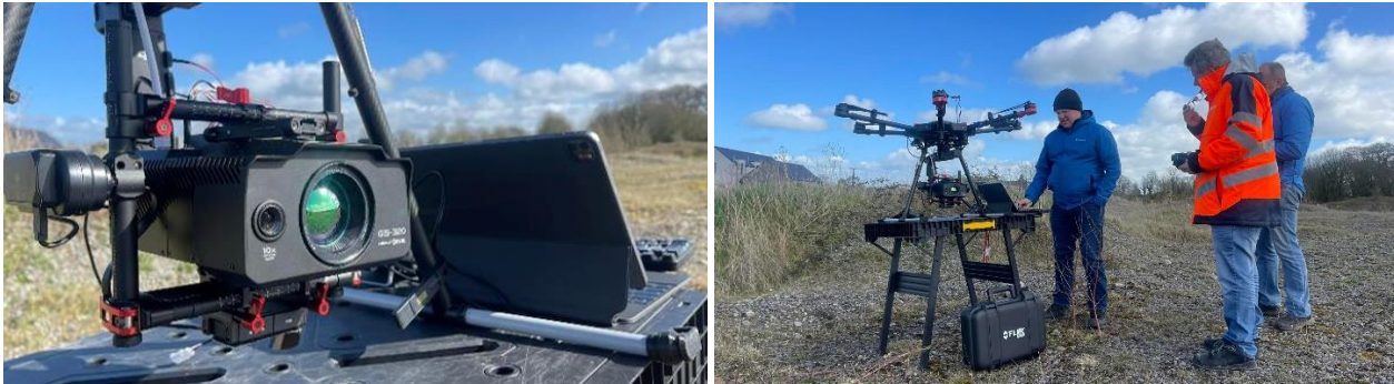
Figure 18: Workswell Methane Sensor GIS-320 mounted on a DJI M600 drone
