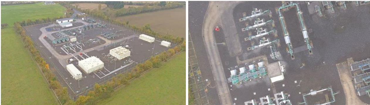
Figure 9: Drone imagery (left image) and 2D photogrammetry survey (right image) of Gormanstown AGI showing high resolution mapping with geospatial information available to analyse
