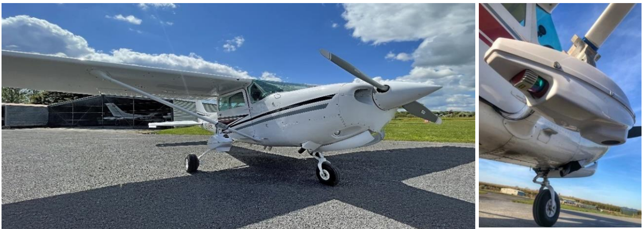
Figure 7: Aerial survey aircraft equipped with LiDAR and RGB sensors (note sensor attached to starboard wing strut)
