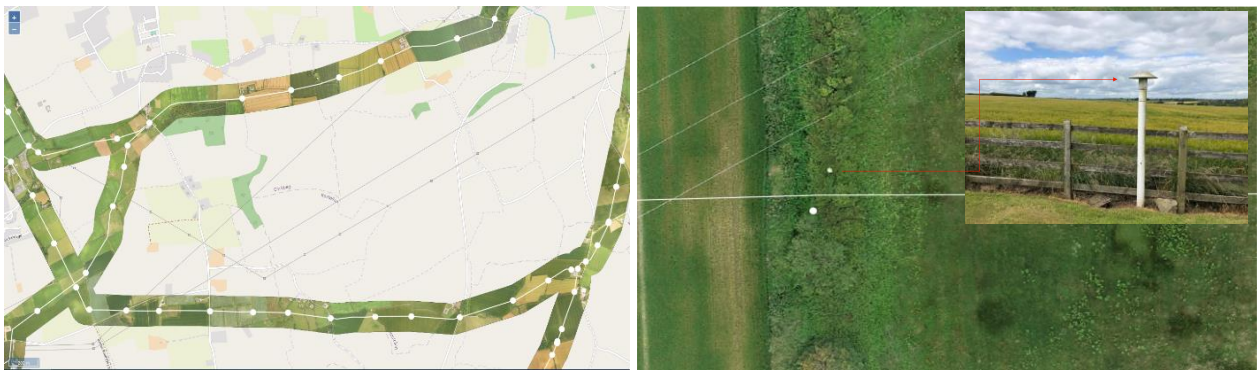
Figure 12: Pipeline route captured by survey aircraft (left image) and zoomed in area of the route with markers clearly visible in the data (right image), ground photo of marker also inserted in right image
