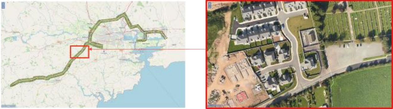
Figure 11: 100km route covered by survey aircraft (left image) and shows zoomed in area with existing pipeline route overlaid and markers clearly visible in the data (right image)
