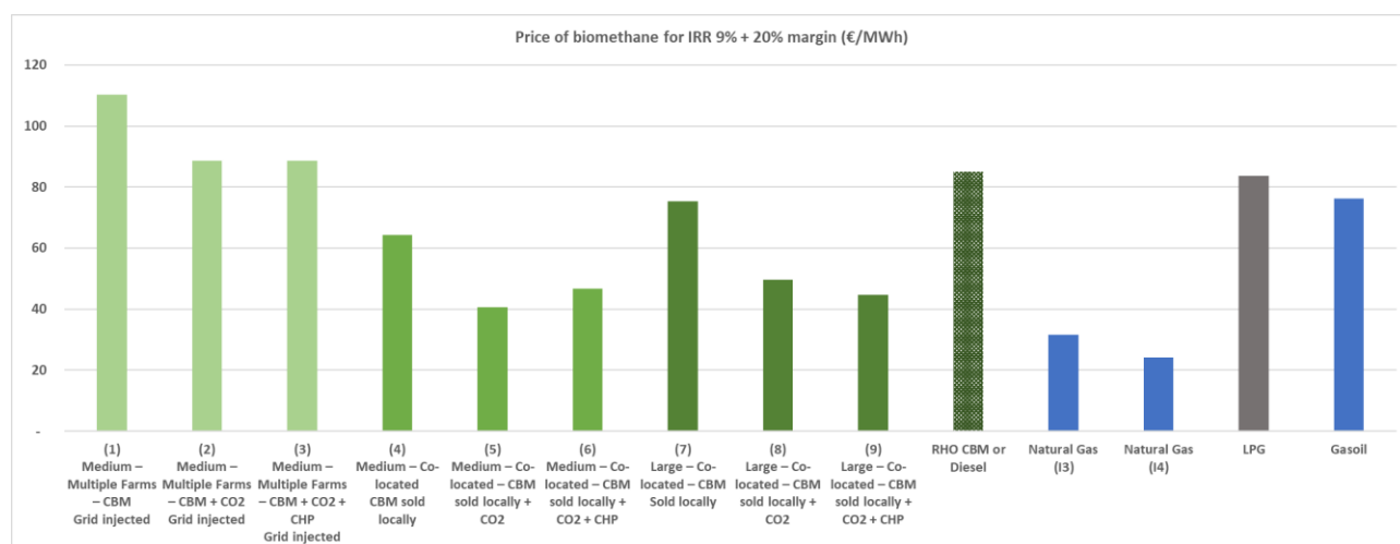
Figure 13: Comparison of CBM value required to achieve 9% IRR with a 20% profit margin, against existing fuels.
