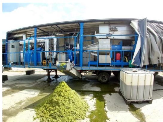
Figure 15: Mobile, containerised grass biorefinery plant. Source: biorefineryglas.eu
