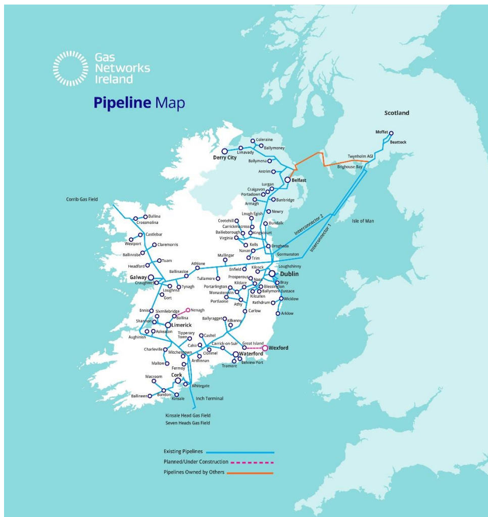
Fig. 2.1 Overview of Gas Networks Ireland Transmission System
