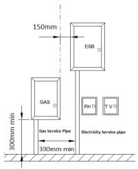
Minimum separation between recessed gas meter and other meters
