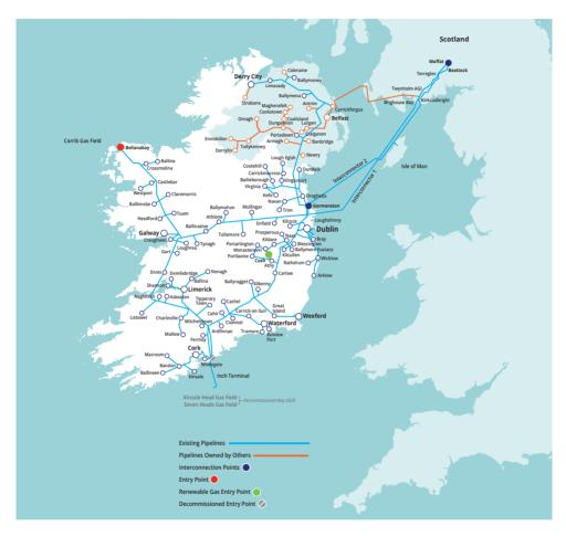
Gas Networks Ireland transports gas in Ireland through a network of steel and polyethylene (PE) pipes. The network operates at pressures between 20 mbar and 85 bar and is split between Transmission and Distribution pipelines.
