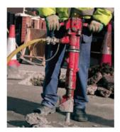
Hand held power tools should not be used directly over the line of a gas pipe, unless the gas pipe has been positively located by hand and a safe working distance has been established.
