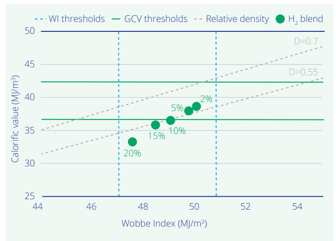
Figure 5. Calorific value and Wobbe Index of natural gas and hydrogen blends from HyTest.
