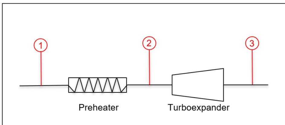
**Figure 1 – Basis Turboexpander Equipment Layout Showing Preheater and Turboexpander**
