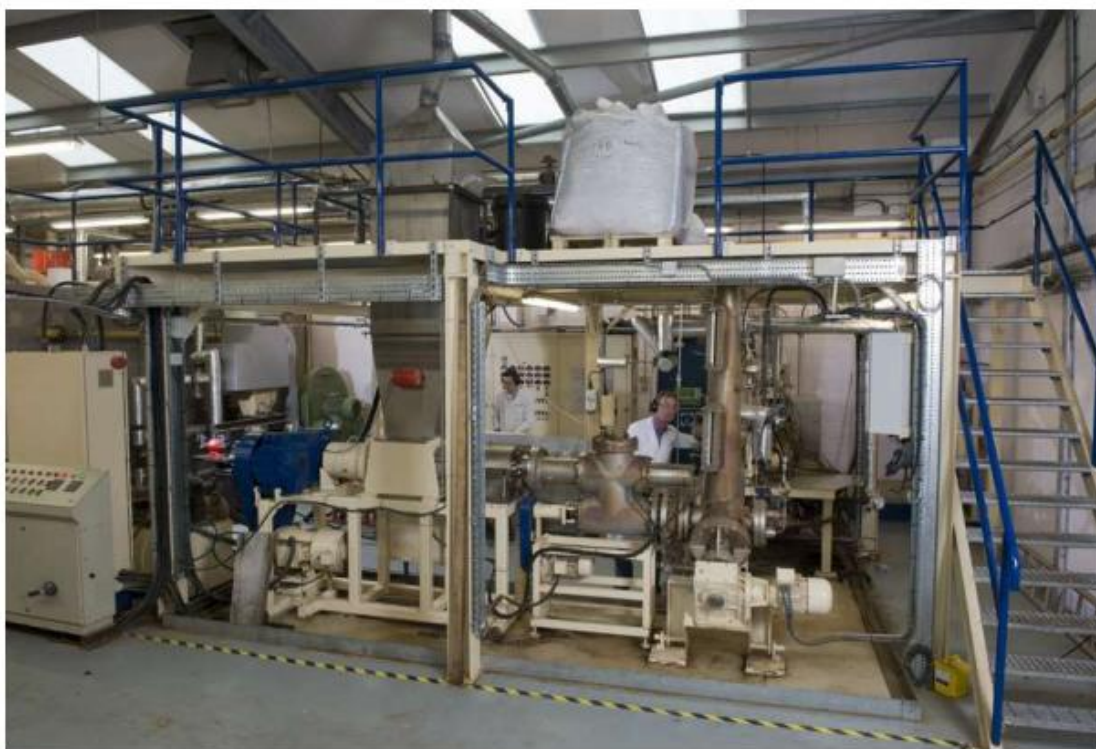
Fig 27 - Pilot scale (Andritz Sprout-Bauer 12 inch - 30.5cm) continuous pressurised disc refining equipment (Bangor University)
