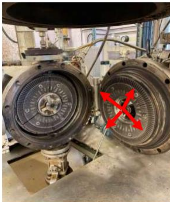
Fig 28 - Refiner plates located inside the refining zone (Note: left plate rotates when operating; right plate is stationary; arrows indicate direction of travel of the biomass through the plates once it exits the digester)
