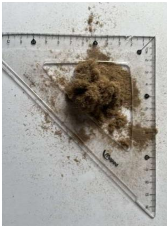
Fig 35 - Willow fibres produced during pilot scale continuous pressurised disc refining trials
