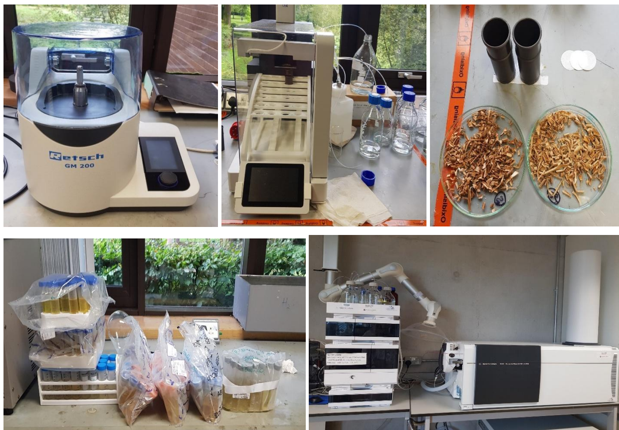
Fig 17 . Equipment used for extraction and analysis (from left to right – Retsch Mill, CEM EDFGE, samples and sample holders, extracts, LC-MS-QToF)
