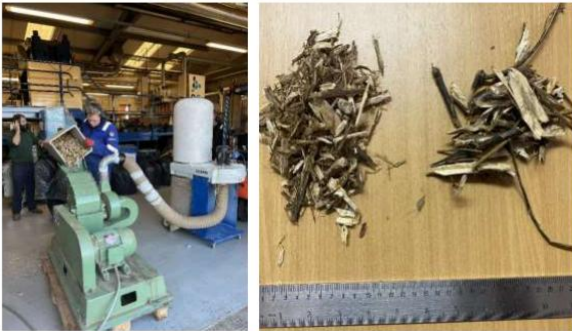
Fig 29 - Hammer milling (a) to reduce particle size of the 'raw willow' (b) compared to the starting material (c)
