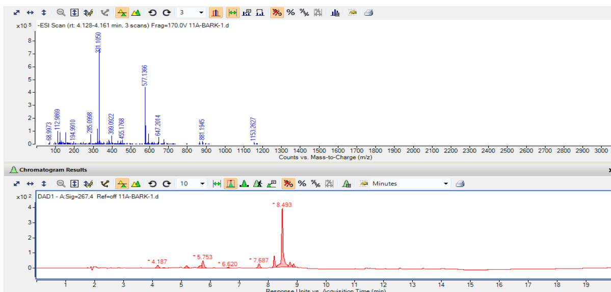
Fig 21 – Example of UV chromatogram of salicin in willow bark extract (below) and m/z fragmentation of peak identified as salicin
