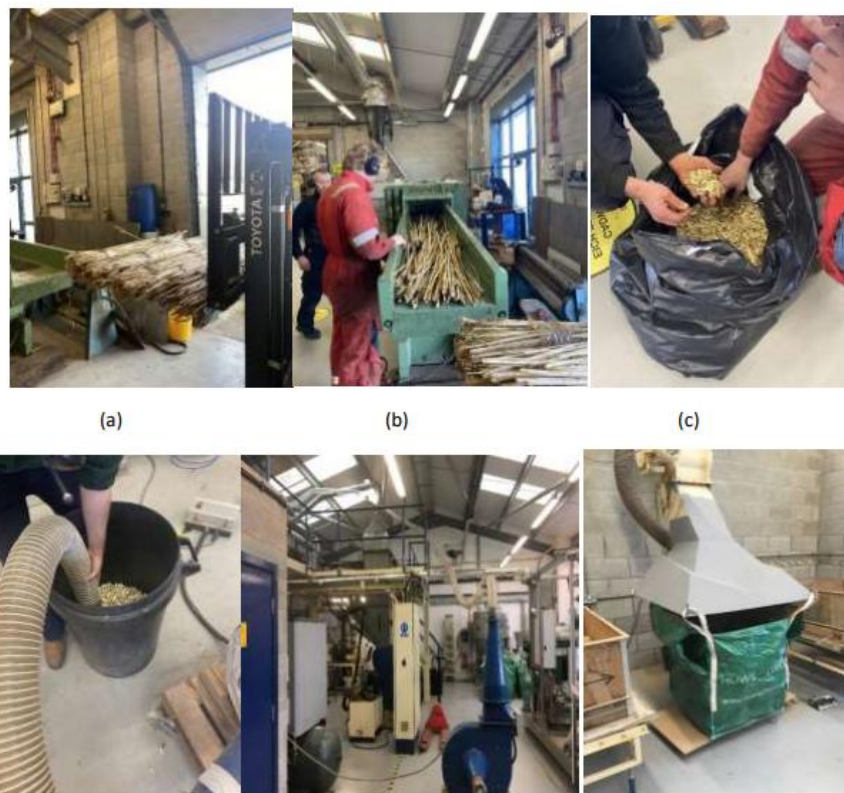
Fig 31. Chopping and drying of harvested willow rods prior to storage and downstream processing.
