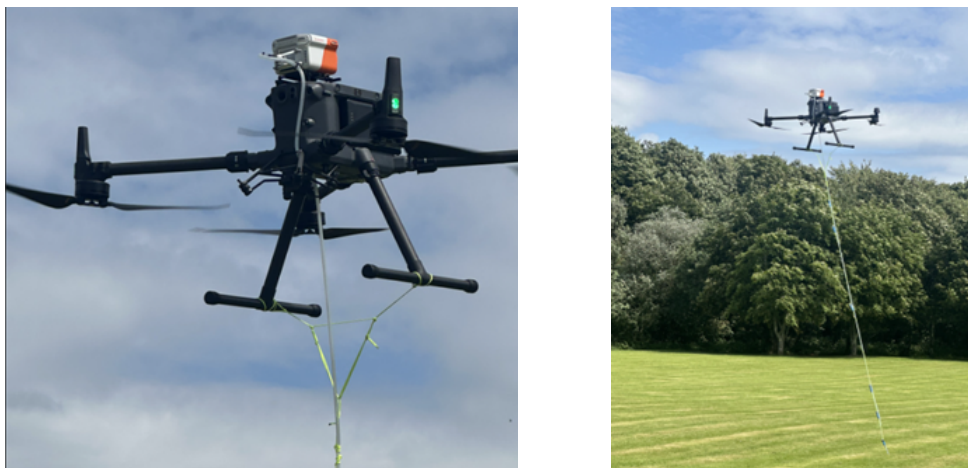
Figure 3: DJI Matrice 350 UAV with Methane gas sensor and sampling hose.
