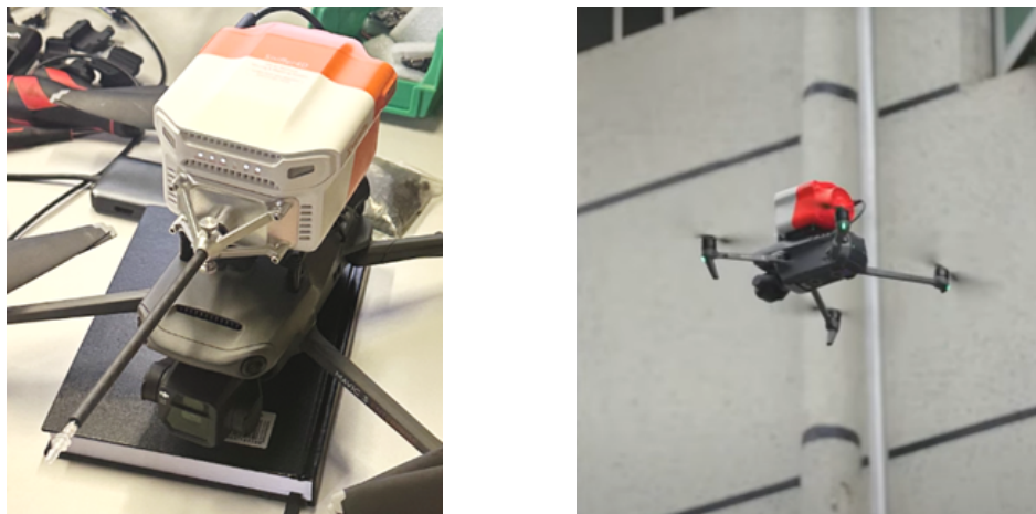
Figure 2: DJI Mavic 3E with Methane gas sensor mounted.
