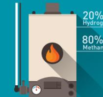
Modern gas boilers and appliances can accommodate a methane/Hydrogen blend of up to 20% Hydrogen. Consumers should anticipate Hydrogen to be first blended into the NI Gas Network from the middle of this decade.
