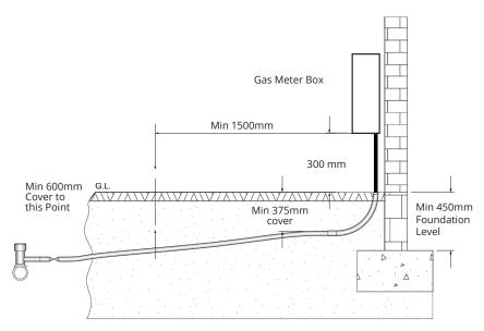
Figure 22: A minimum cover of 375mm and minimum foundation of 450mm are necessary
