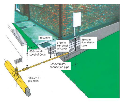
Figure 21: Connection pipe with preformed bend attached to Mains showing minimum level of Cover and Foundations required.
