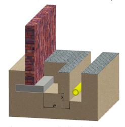
Figure 45: Proximity of walls to foundation
