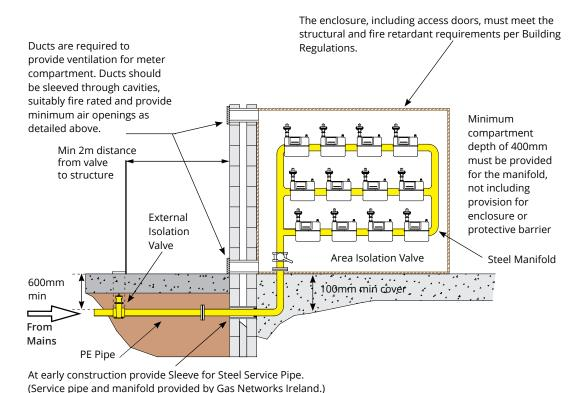
Figure 28: Multiple meter within a building
