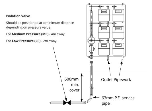
Figure 27: Diagram of pipework and meter cabinet
