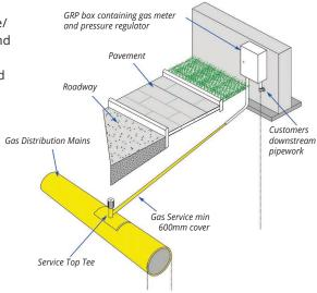
Figure 1: Connection from Gas Main to Residential Meter Box
