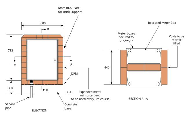
Figure 19: Meter box in pillar enclosure
