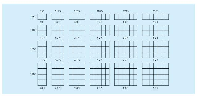
Figure 42: Internal Building Dimensions for Various Meter Bank Configurations
