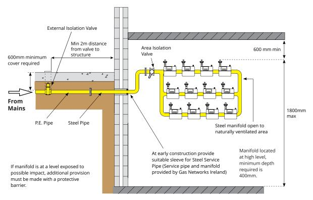
Figure 31: Meters in underground car park / open basement area
