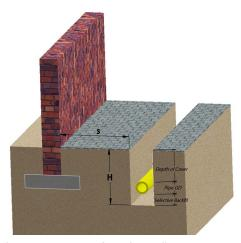
Figure 44: Proximity of trench to walls
