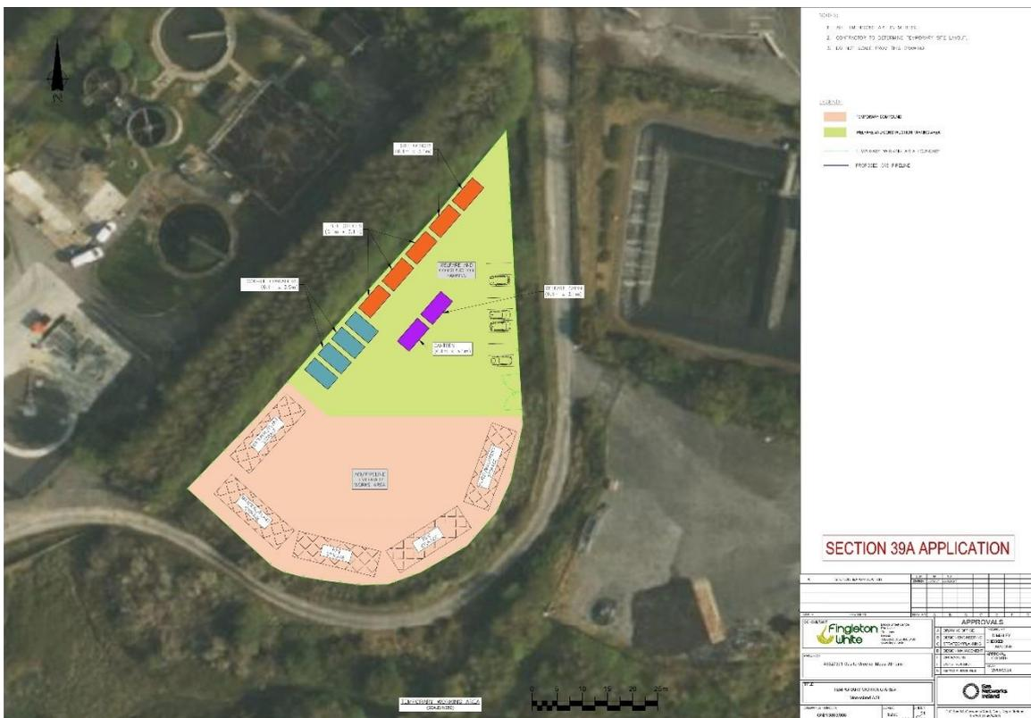
**Figure 4.6** Proposed AGI Temporary Works Area Layout (Fingleton White Ref: GNI-13803-008-04)
