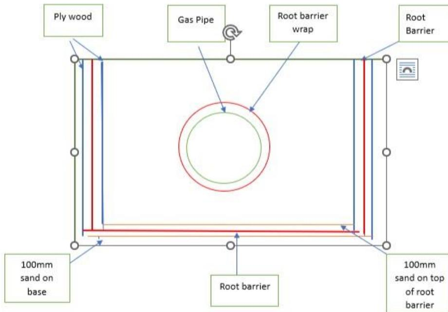
**Figure 5.1: Side Profile of Root Barrier Placement**
