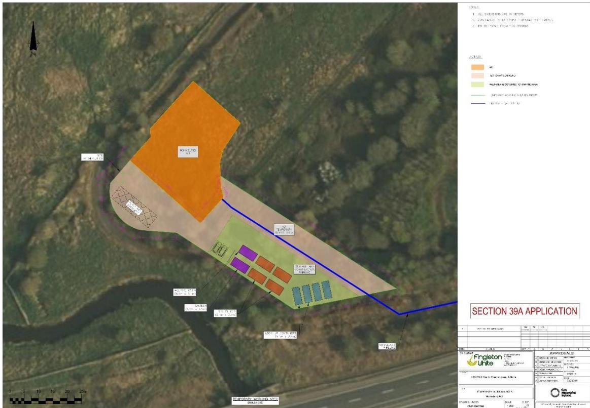
**Figure 4.4** Proposed AGI Temporary Works Area Layout (Fingleton White Ref: GNI-13803-008-02)
