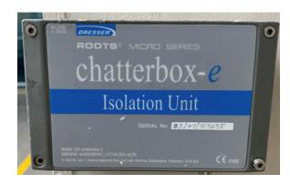
The chatterbox is powered by two 3.6 volt lithium batteries, which have a potential working life of up to 10 years. The output from the chatterbox is opto-isolated with a pulse width of 220 ms capable of accepting 20 V and a maximum load current of 130 mA.
